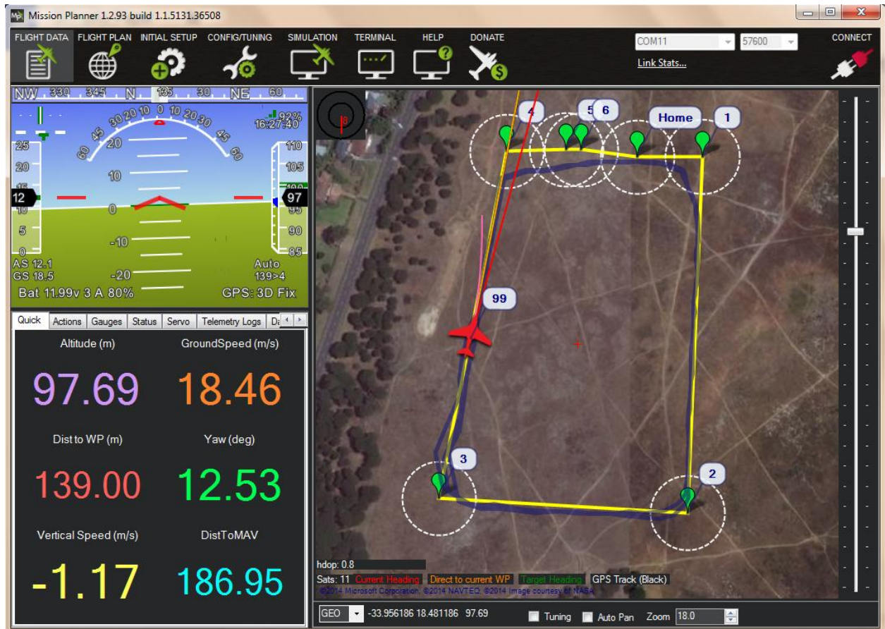
Figure 2. GCS Software Mission Planner showing an aircraft flying an auto mission
