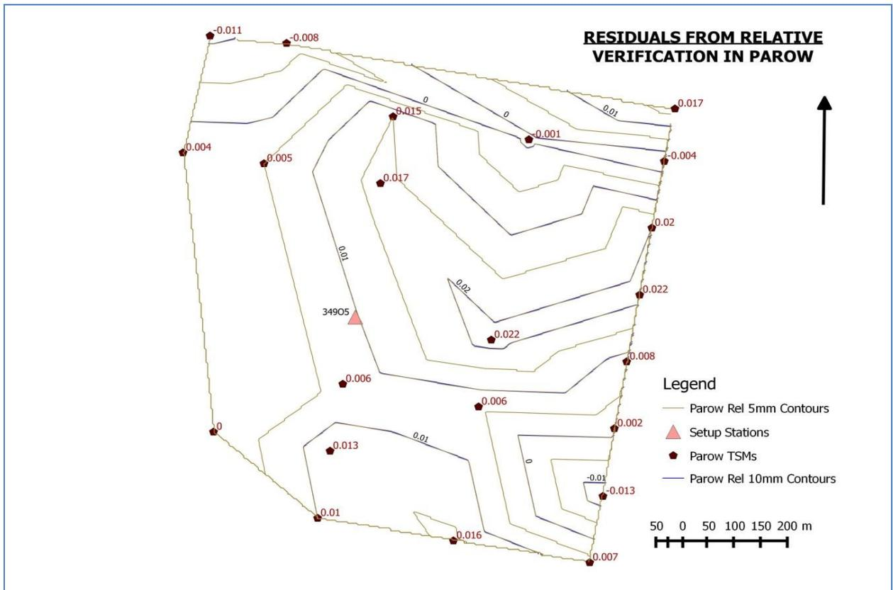
Figure 6. Contours showing residuals from relative verification in the Parow study area.
