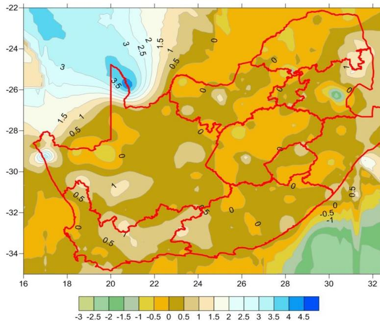
Figure 2. Differences between published orthometric heights of trigonometrical beacons and orthometric heights using the SAGEOID2010 (metres) (Wonnacott & Merry, 2011)
