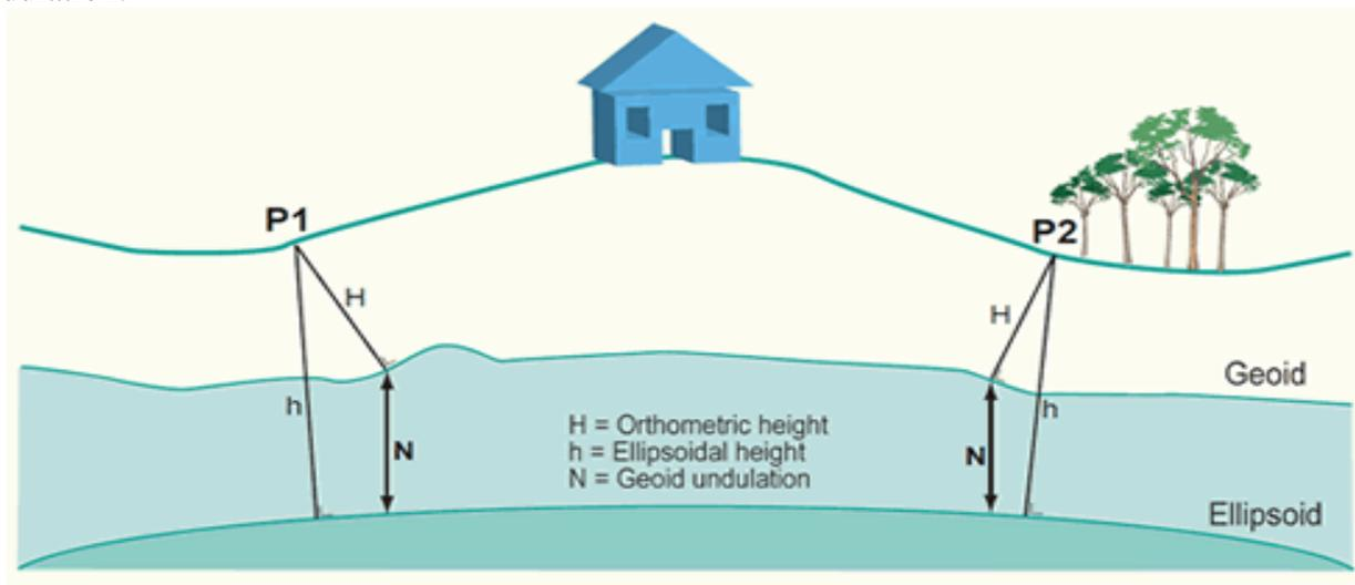
Figure 3. Relationship between the ellipsoid and the geoid
