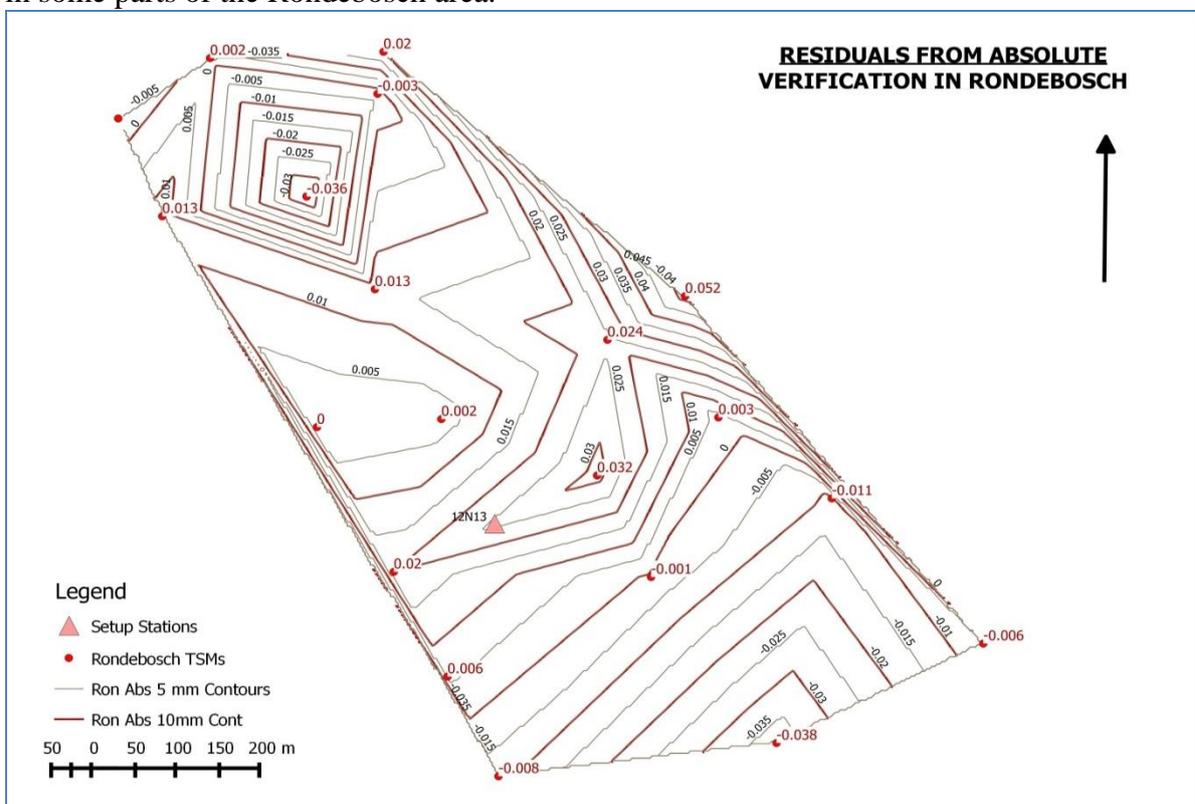
Figure 7. Contours showing residuals from absolute verification in the Rondebosch study area.
