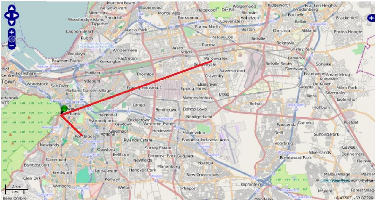
Figure 4. Sensor map showing the lengths of the baselines from the nearest CORS at Mowbray.
