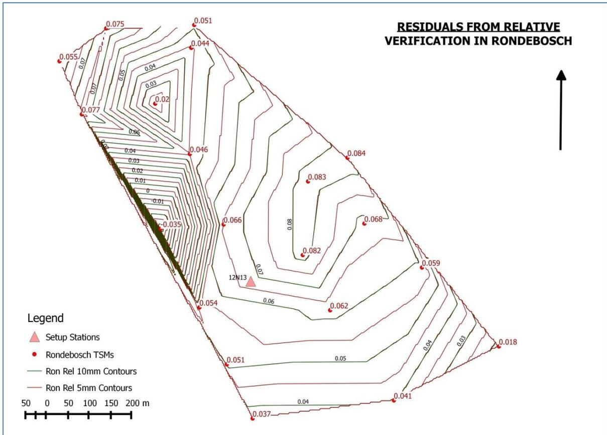
Figure 8. Contours showing residuals from relative verification in the Rondebosch study area.
