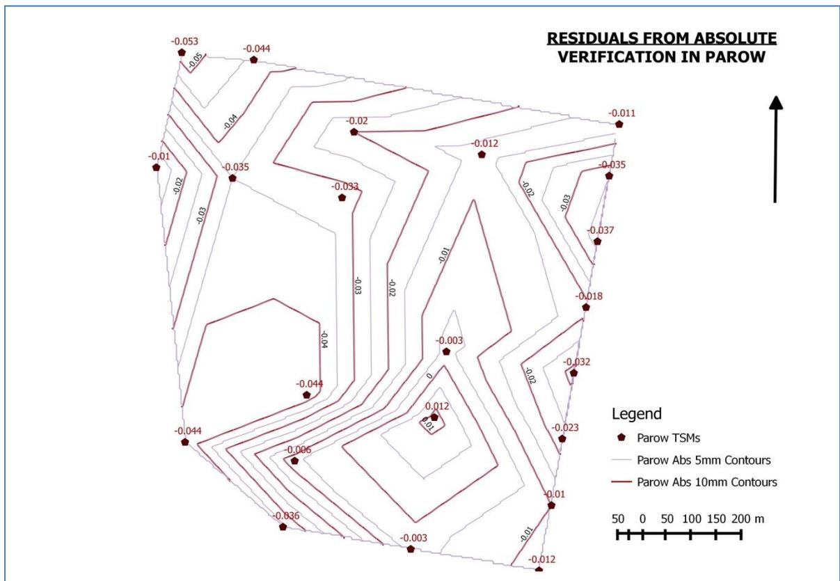
Figure 5. Contours showing residuals from absolute verification in the Parow study area.
